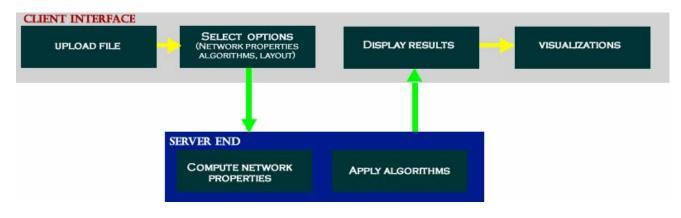
Figure 1: Architecture and the flow of computation through the envisioned system.
