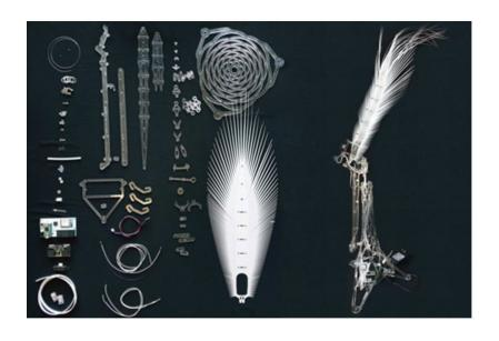
Amatria Dendrites, on display in the Luddy Hall Visualization Lab (room 4012), are pieces of living architecture. Each comprises one light sensor (the eye) and actuators such as lights and a strand of shape memory alloy that makes the sculpture move. Software controls the sensor and actuators. Dendrite fields were built in the 2017 ISE Summer camp. See below for events and activities where you can build or view dendrites.
