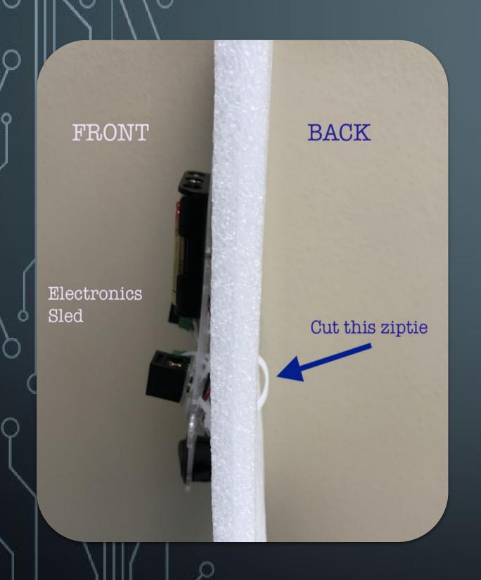
The electronics sled comes almost fully assembled. To finish assembling this section, there are only three steps:
