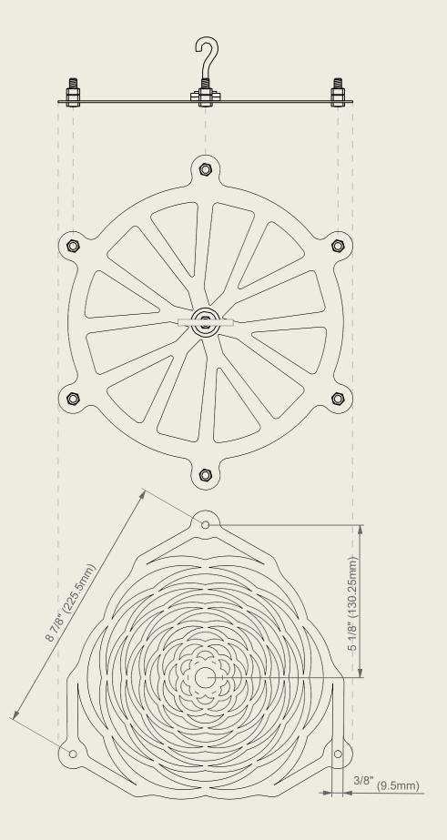
Cutting Pattern and Forming Plat 3mm Acrylic Fastened to Steel Frame
