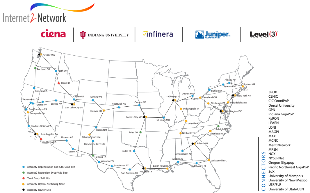
Figure 3.1: Map of the Internet2 network backbone, which connects hundreds of colleges, university, and other research institutions with high-speed fiberoptic links. The black dots indicate the core router nodes that generate network flow records. (Map courtesy of Internet2 network.)
