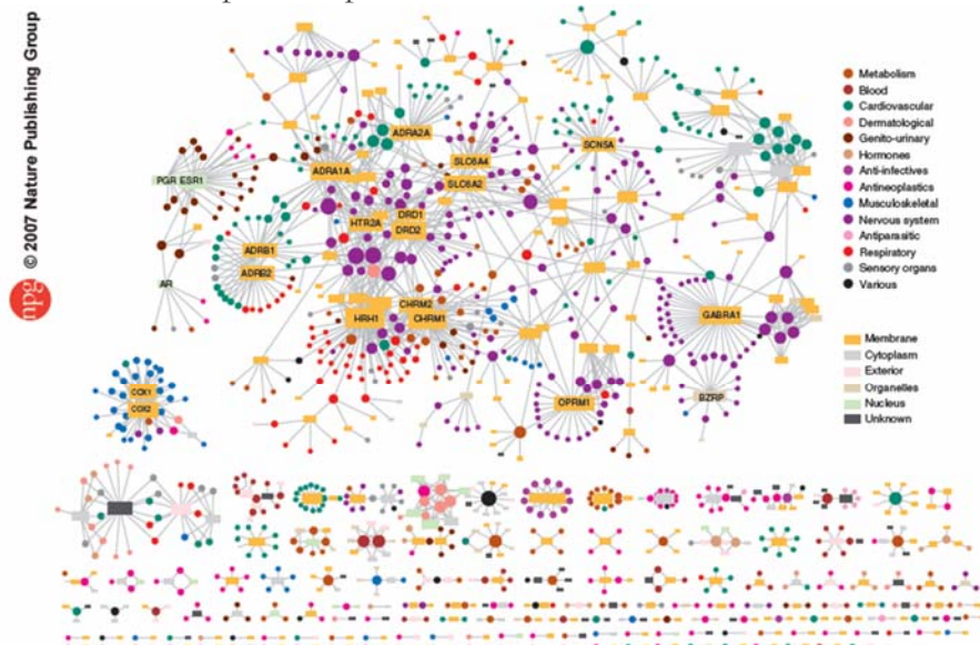
Figure 2 Drug-target network (DT network). The DT network is generated by using the known associations between FDA-approved drugs and their target proteins. Circles and rectangles correspond to drugs and target proteins, respectively. A link is placed between a drug node and a target node if the protein is a known target of that drug. The area of the drug (protein) node is proportional to the number of targets that the drug has (the number of drugs targeting the protein). Color codes are given in the legend. Drug nodes (circles) are colored according to their Anatomical Therapeutic Chemical Classification, and the target proteins (rectangular boxes) are colored according to their cellular component obtained from the Gene Ontology database.
